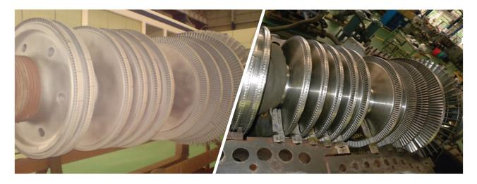
Based on this a **10 stage** rotor was redesigned to a **11 stage** rotor.
