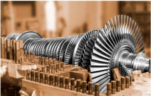
15.6 MW Turbine during mechanical steam run test at the shopfloor
